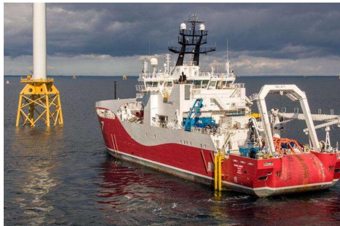
*Cable laying vessel (source : Seaway 7)*
