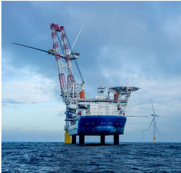
*Wind Turbine Installation Vessel - Jack-up vessel (Source : Jan de Nul)*
