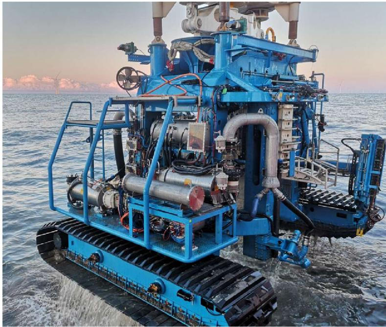
*Mechanical trencher (Source : LDTravocean)*
